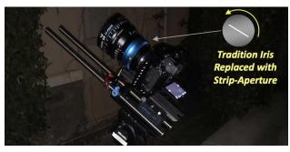
The rotating synthetic aperture (RSA) architecture is an expression of this optimization. Its strip-aperture
